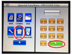
**2.** Press the Recipe button, enter the pin code "5678", then press the button
