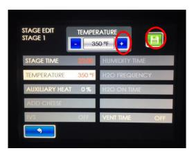
**5.** Press "Temperature", then change to "360" utilizing the "+" button, then press the green 'save' button in the upper right corner. When complete, press the back arrow.
